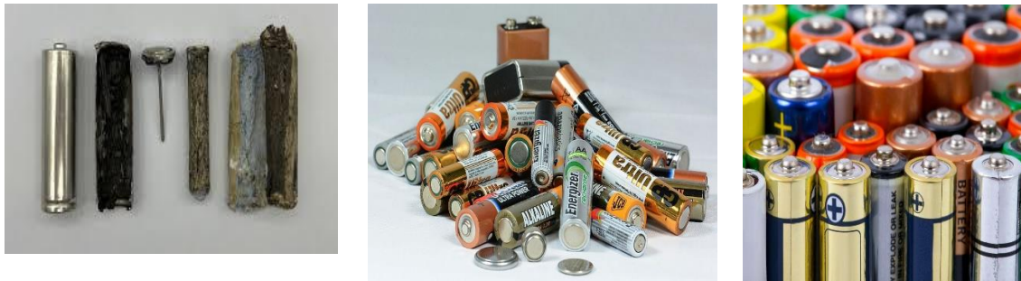
Figure 1 Presentation of Zinc Battery Envelopes
